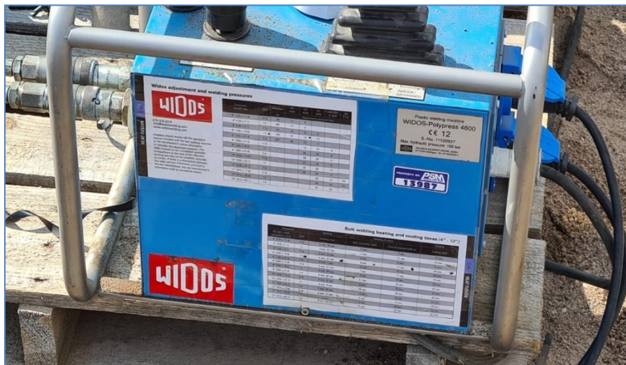
Figure 35 – Widos-Polypress 4600 Fusion Machine
