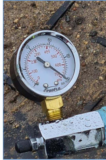
Figure 16 – 100PSI for 24 hours
