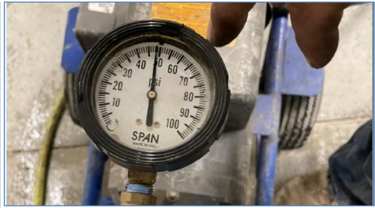
Figure 57 – Purging Pressure from Pump. No documentation provided for GPM, although a meter is present in Photos
