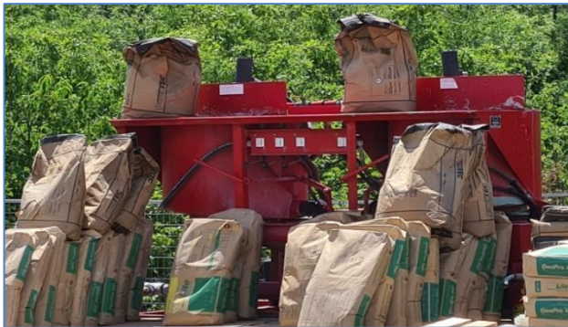
Figure 20 – The dual tank grout pump with materials staged for mixing
