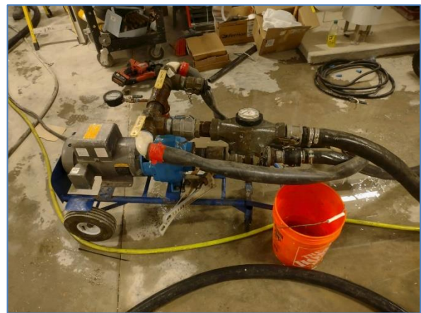
Figure 55 - Goulds Water Technology 50SPM20F Purge Pump w/pressure and flow meters.
