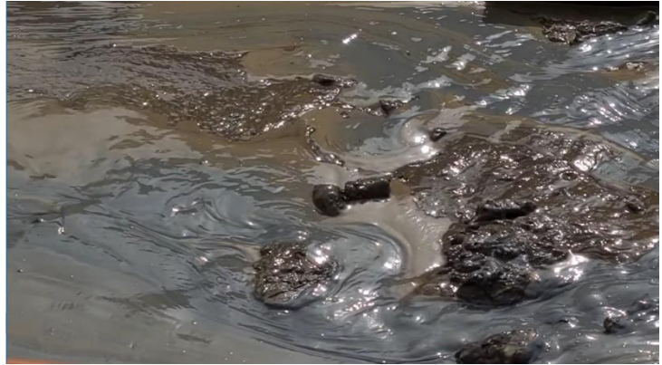
Figure 25 - Evidence of Graphite in Grout.
