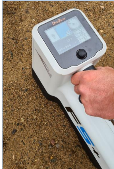
Figure 18 - Locating w/ DigiTrak F5+
