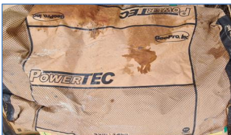
Figure 6: Graphite Grout Enhancer
