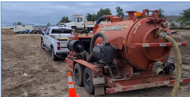
Figure 27 - Mud pumps used to manage grout and mud
