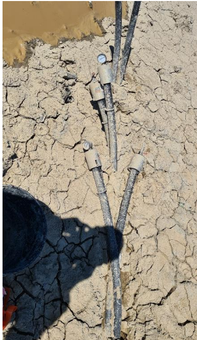
Figure 15 - A Row of Loops Under Pressure Test for 24 Hrs after Grouting
