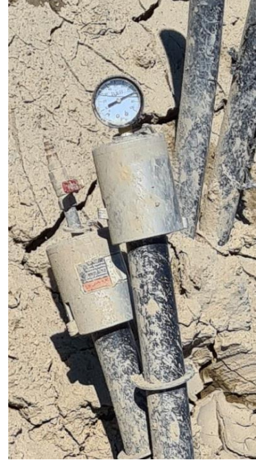
Figure 16 - Loops Pressure Tested to 80PSI
