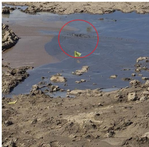
Figure 24 - Hydraulic Pressure Breakthrough on Pond Bottom. Note Evidence of Graphite in Grout.
