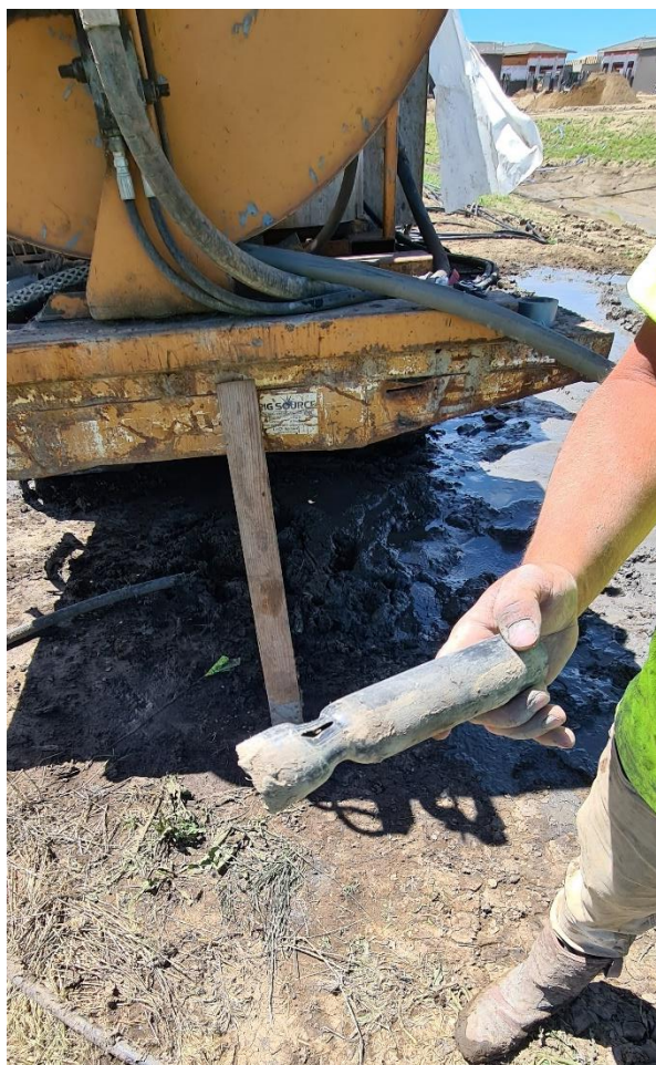
Figure 20 - Tremie Pipe Separation. Borehole Angle and Resistance Prevent Successful Grouting of Early Borehole
